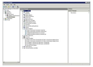
Figure 6 Each CNA port is represented as an HBA and a NIC to Windows Server
